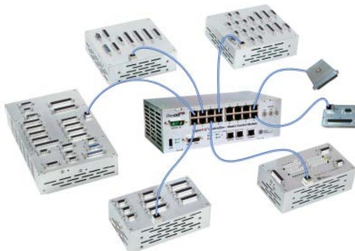
The **FUSION Controller** is the newest member of the SuperIO family that is a 4 port CM “fused” with a 24 slot RIM into a single unit. FUSION units can also connect with up to 4 additional RIMs. An example network diagram with FUSION design is shown in Figure 2.
