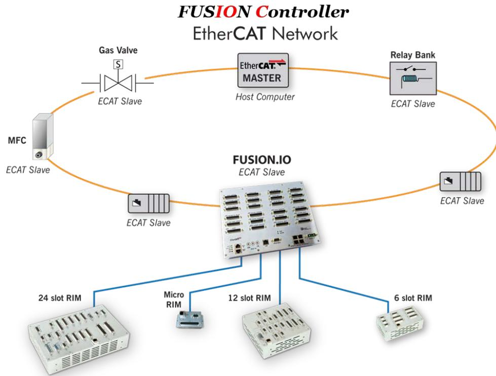
RIMs can be customized with a variety and number of Input/Output (I/O) cards as shown in figure 3.
